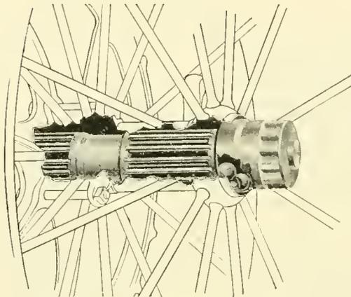
Note ball and roller bearings on main axle —
