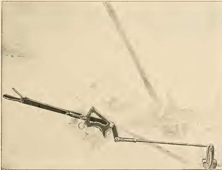
Showing tilting lever, quadrant and connections
