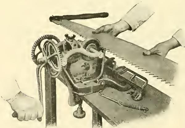
Gumming a cross-cut saw
