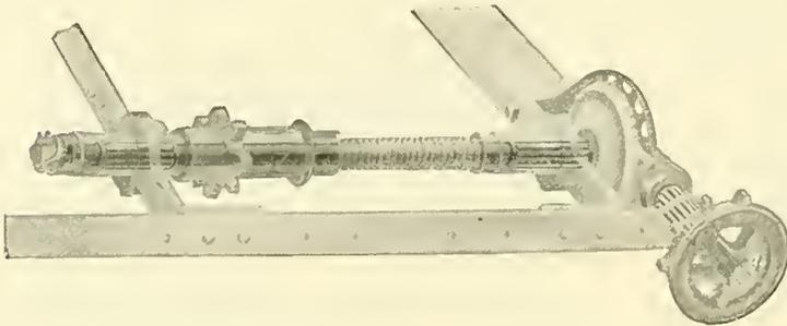
Main gear shaft and crank shaft with frictionless ball and roller bearings
