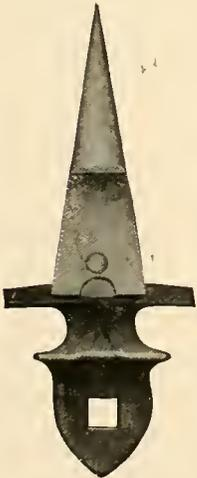
Note that the ledger plate extends back of the finger bar
