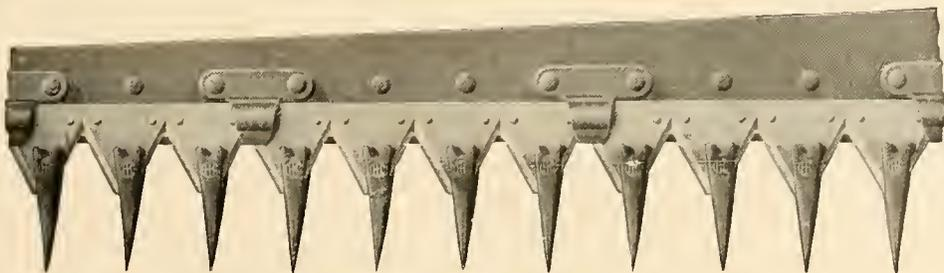
Section of New Ideal mower cutter-bar
