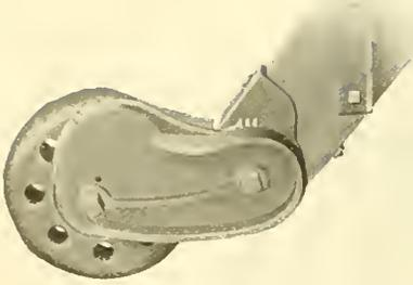
Ground wheel adjusted for bringing rakes close to ground
