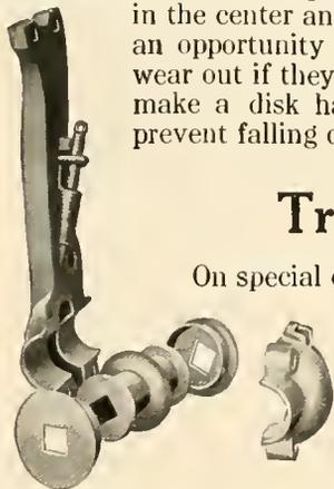
The center ring projection on the bearing relieves the end of the bearing of end thrust
