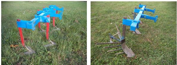
Images 16 & 17: The disconnected toolbars for quickly changing to from for example: hoeing to hilling.
