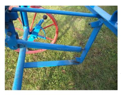
Image 22: Showing the end of the steer bar, which can be locked in the holder. The holder is the lower triangle in the corner of the frame. The weight of the toolbar pushes it into a locked position (see Image 11 for the transport position).
