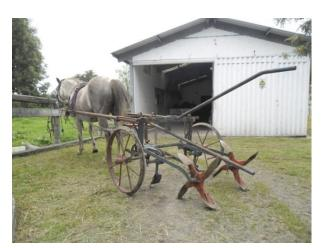
The plant hole makers can be set at 4 different potato row widths:
