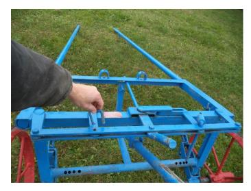
Image7: When this pin is pulled out, the tool carrier comes out of transport position. Then the toolbar and wheels both become steerable.
