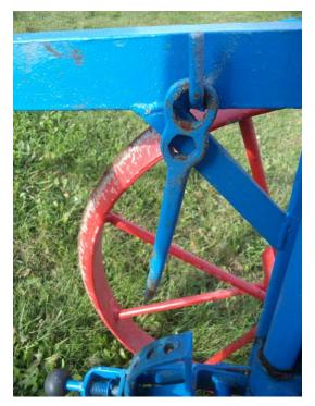
Image 23: Next to the hammer there is also a wrench. For two sizes and the tail is used for the ring bolts.
