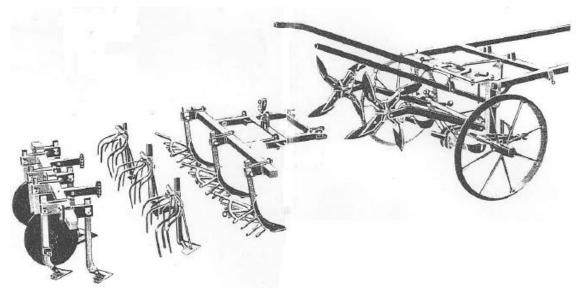
Image 2: Showing different tools that can be attached to the Köckerling.
