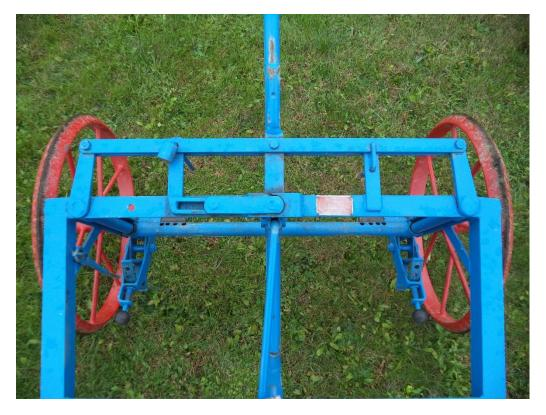
Image 6: The toolcarrier steering system in transport mode.
