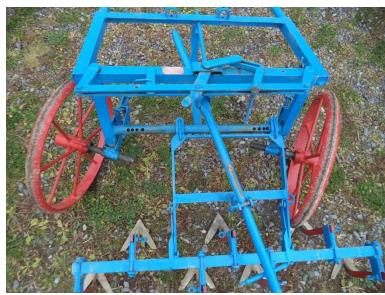
Image 10: a closer look up to the steerage system when steered to the right with wheels and toolbar.
