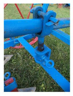
Image 14: The ring bolt can be loosened so the steering bar can be put higher or lower. The vertical round bar has holes in it where the bolt is screwed into.
